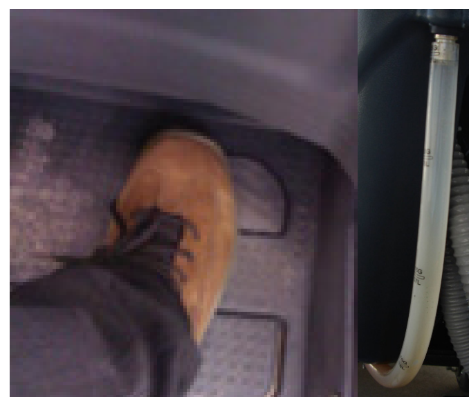
13. Press the forward pedal, select the direction and start operating the machine
