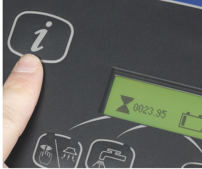
1. Check the battery charge gauge (and if necessary re-charge)
