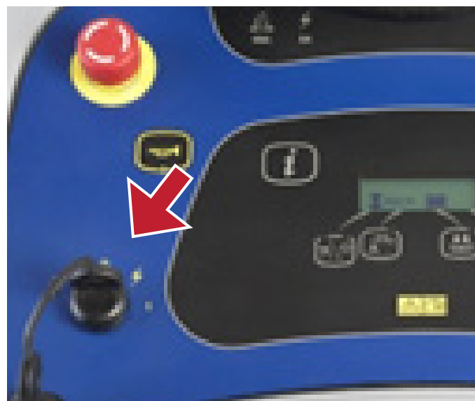
7. Stand on the machine and turn on the key (squeegee lowers automatically)
