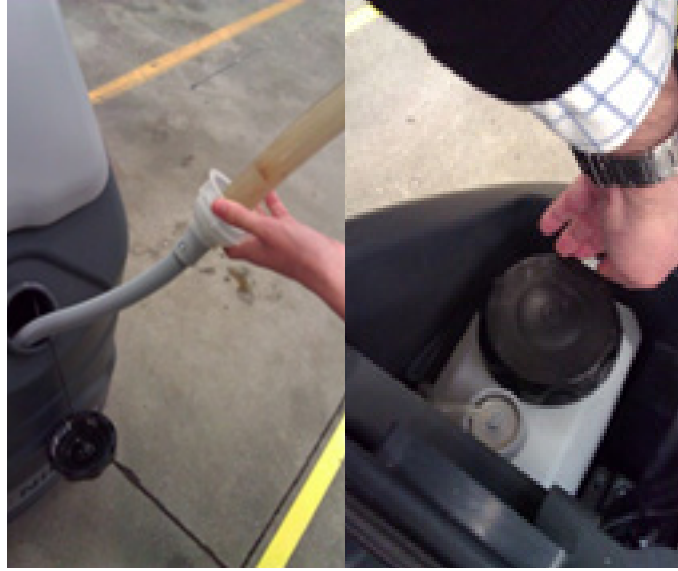
2. Fill-in the tank with clean water. Check if the Ecoflex bottle is well installed (only for machine with Ecoflex)
