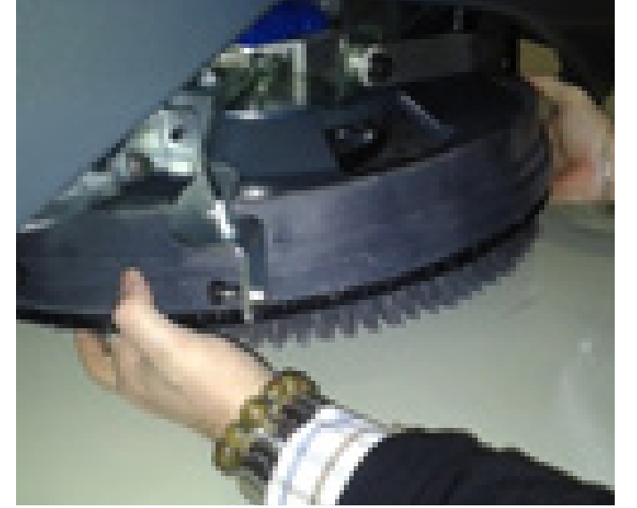
5. Install the brush on the deck
