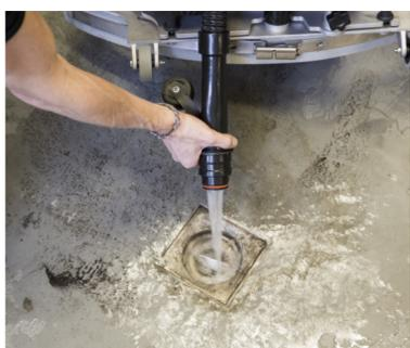
10. **At the end of the work.** Empty the recovery tank with the hose. Then empty the solution tank with the transparent hose
