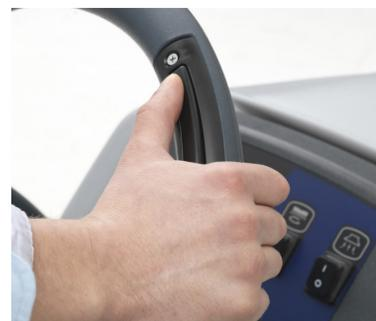
9. Press the handle switch to engage the brush and run the machine
