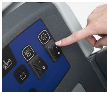
8. Switch on the brush and vac motors to activate the machine
